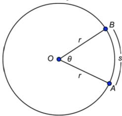
Notice that  $\angle AOB$  cuts off or determines an arc  $\overrightarrow{AB}$  that has length s. The radian measure of a central angle, often denoted by the Greek letter theta ( $\theta$ ), is defined to be the ratio of the arc length to the length of the radius. So the radian measure of  $\angle AOB$  is given by:
